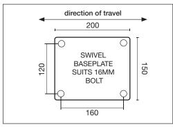
Standard baseplate dimensions & drilling patterns for Single Wheel EHP castors
