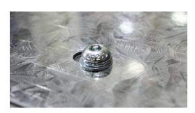
Repeat step 8 for each of the threaded holes on the base of the tub until all are fully tightened.
