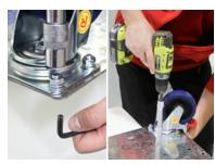
Using a 13mm socket and a 5mm allen key tighten all of the fasteners on the mounting plate.
